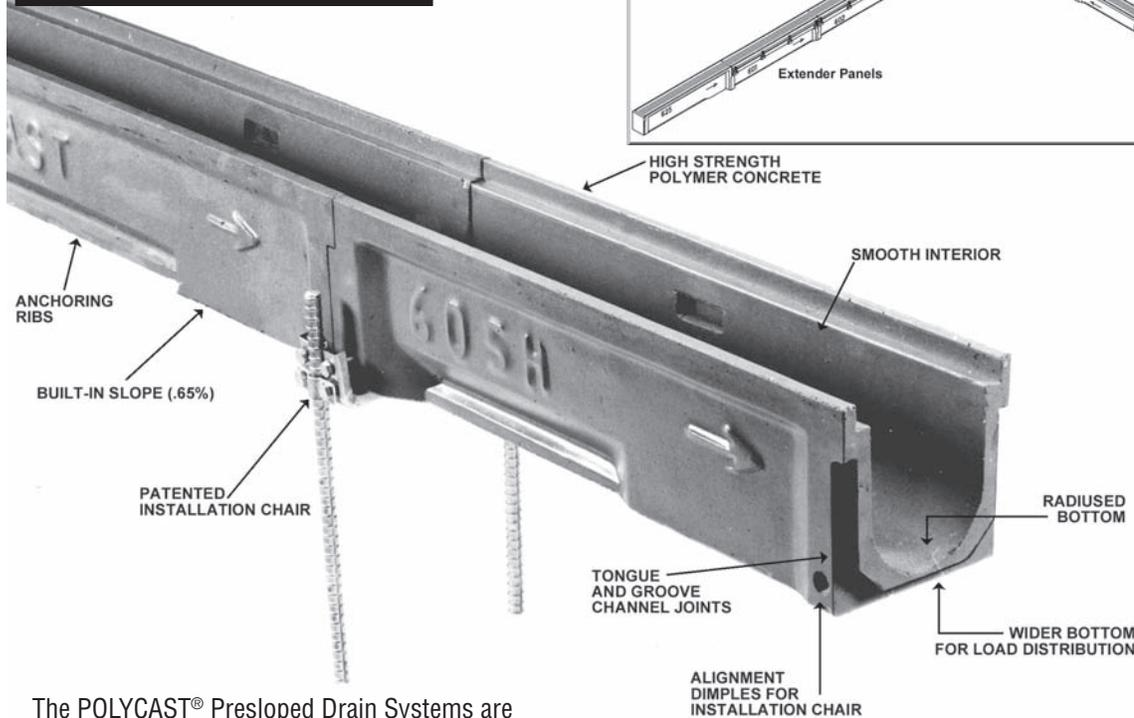
The POLYCAST® Presloped Drain Systems are designed for a variety of applications, both indoors and outdoors. POLYCAST® is made of a high strength, chemical resistant, composite material. As a result, POLYCAST® drains offer a high degree of chemical resistance and have a water absorption value of less than one percent (ASTM C140).
