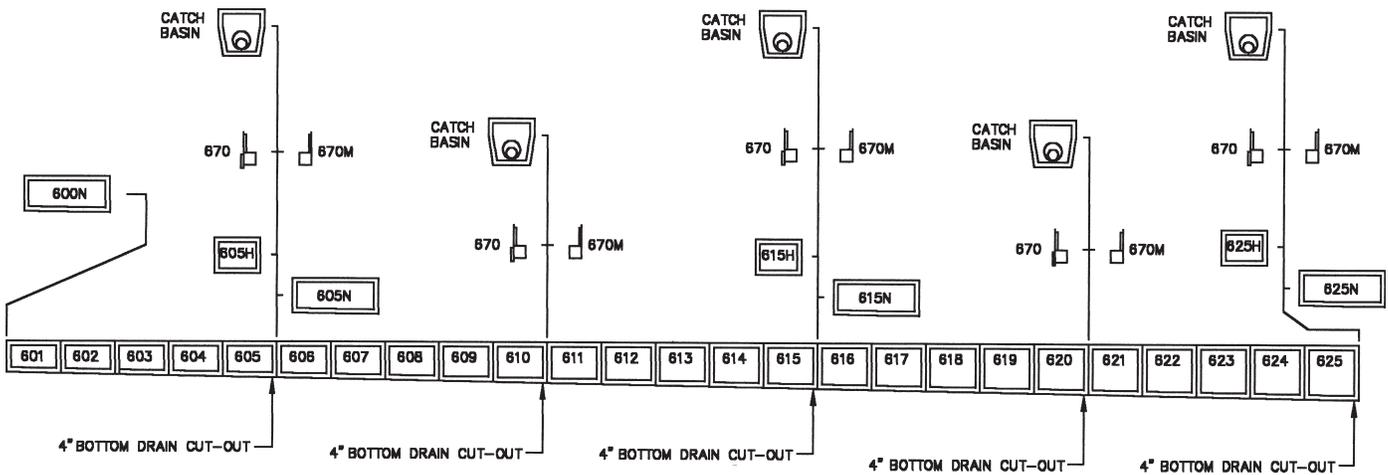
NOTE 1: All half and neutral channels have bottom cut outs. NOTE 2: All half and neutral channels accept the corresponding end caps.
