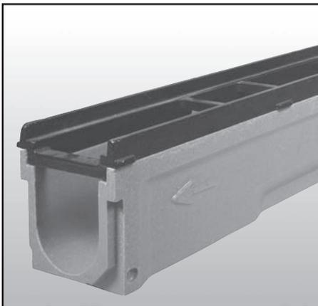
The 700 Series assembly consists of HARDNOSE cast iron frames inlaid on the top of the conventional 600 Series polymer concrete Channel and fitted with either Gray Iron or Ductile Iron Slotted Grates (described in more detail on page 27). Uses grate hold-down device Part. No. DA0642BH.
