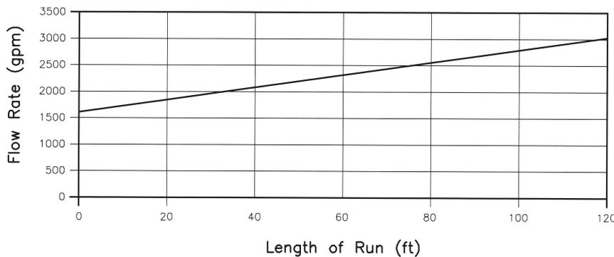
**Flow Capacity with 1% Continuous Built-in Slope**
