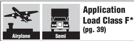
\* Class F grates with spans of 12" or more are rated for a 120,000 lb. wheel load over a 10" x 20" footprint per ASTM C-857.
